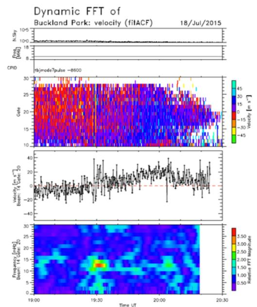
BPK range-time plot (left), beam 14 1920 – 2000 UT, showing Doppler oscillations over  $\pm 40$  m/s, and (right) FFT over 1900 – 2030 beam 14, range gate 20 (~ 500 km SE of BPK) with oscillations around 13 mHz.
